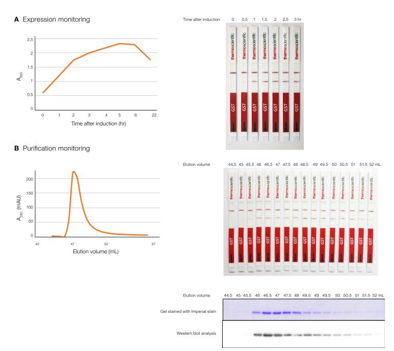
Figure 4. Monitoring expression and purification of GST-GFP using the Pro-Detect Rapid GST Assay Kit.
