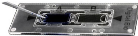
**Note:** Each chamber in the Countess™ Cell Counting Chamber Slide has a 10-µL sample capacity. Do not overfill the slide chambers.
