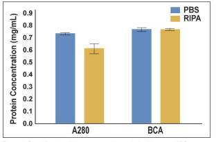
Figure 4: Quantification of the same protein sample in either  $0.5 \times PBS$  or  $0.5 \times RIPA$  buffer. Quantification was performed using both A280 (blank performed using the appropriate buffer) and the BCA colorimetric assay (standard curve prepared using the same buffer). *Note that the A280 measurement of the sample in RIPA buffer was not only inaccurate, but also showed poor reproducibility.*
