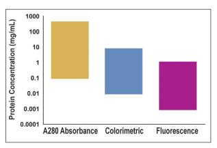
Figure 2: Comparison of the approximate dynamic ranges associated with the various protein quantification methods using a NanoDrop spectrophotometer or spectrofluorometer.
