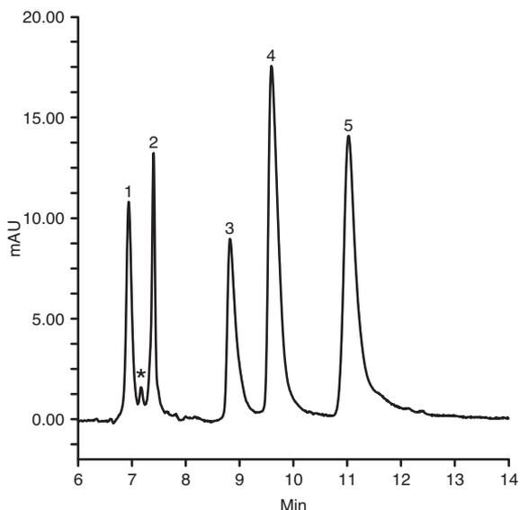
Figure 1: UV chromatogram for five proteins separated on an Accucore 150-C4, 150 mm x 75  $\mu$ m nano HPLC column (blank injection subtracted to compensate for the change in baseline with acetonitrile concentration). The proteins are listed in Table 1, \* indicates an impurity from carbonic anhydrase.
