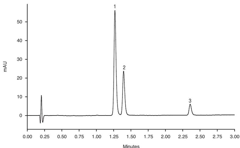
Figure 1: Chromatogram for ketoprofen 1, naproxen 2, and ibuprofen 3, separated on an Accucore Polar Premium 2.6  $\mu$ m, 50 x 2.1 mm column.
