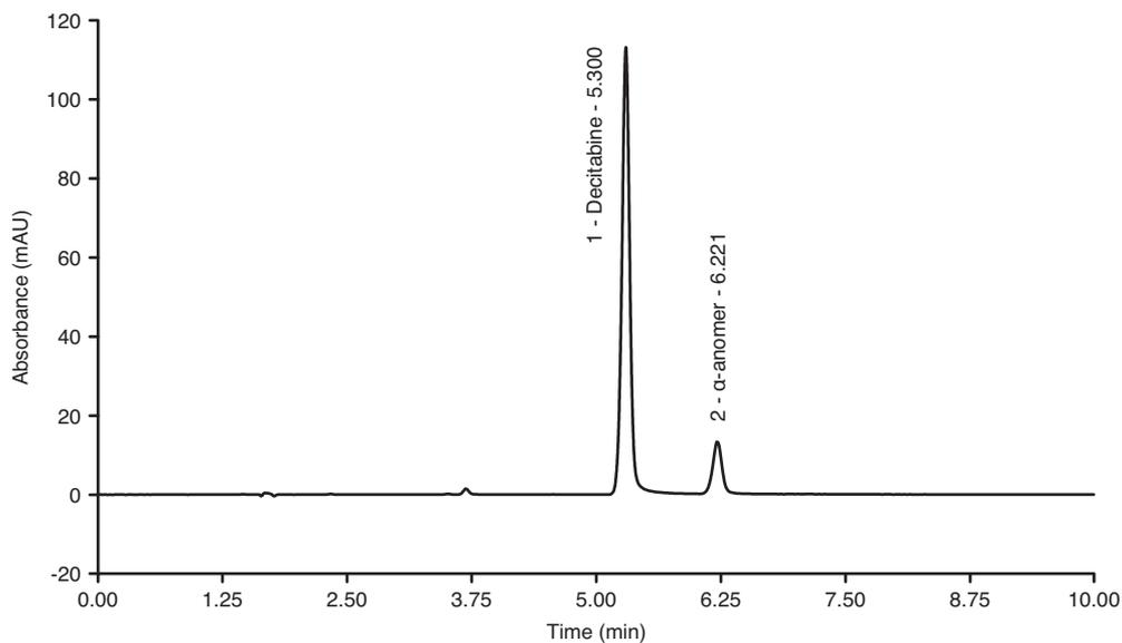
Figure 2: Chromatogram of decitabine and its α-anomer impurity
