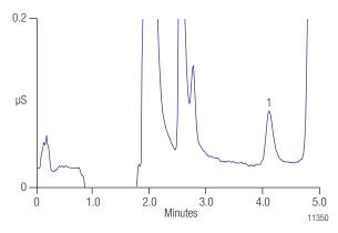
Figure 5. Bromate in the presence of 200 mg/L of chloride, carbonate, and sulfate.
