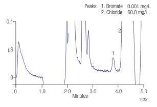
Figure 6. An ozonated drinking water sample is spiked with 1.0  $\mu$ g/L of bromate.
