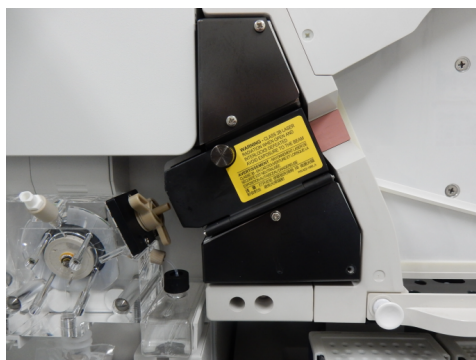
Figure 33 Detection cell cover (front view, door open)
