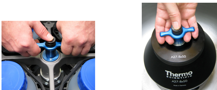
Figure 25: Holding the rotor during removal
