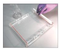
4. Remove the end gates, place the UVT gel tray in the buffer chamber, add buffer, load samples, and run the gel.
