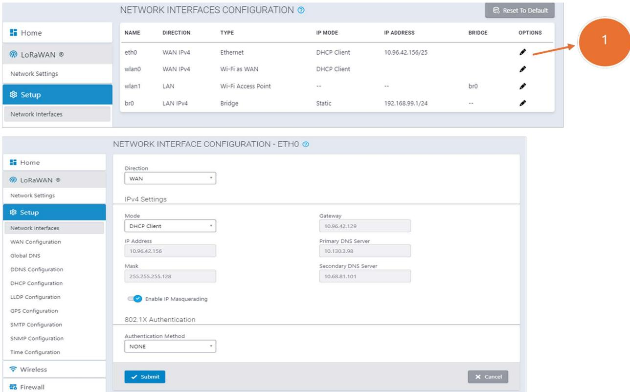
**Figure 42. Ethernet Configuration**
