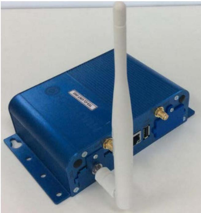
**Figure 6. Attach Smart-Vue Pro LoRaWAN Antenna to connector labeled “RF”**
