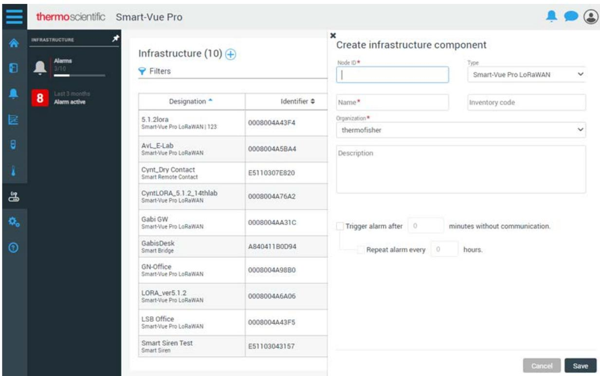
Figure 47. Add Smart-Vue Pro LoRaWAN details in Infrastructure
