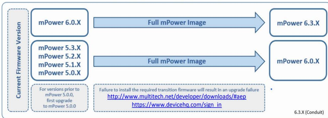
Figure 38. Firmware Upgrading Process
