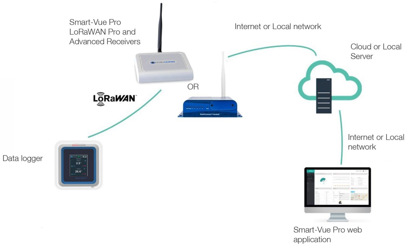
**Figure 5. Receiver connecting Smart-Vue Pro Quatro/Duo data logger to the Cloud**
