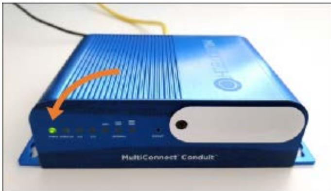
**Figure 9. Power indicator remains on when receiver is ready to use**
