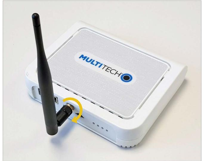
**Figure 7. Attach Smart-Vue Pro LoRaWAN Antenna to connector labeled “RF”**
