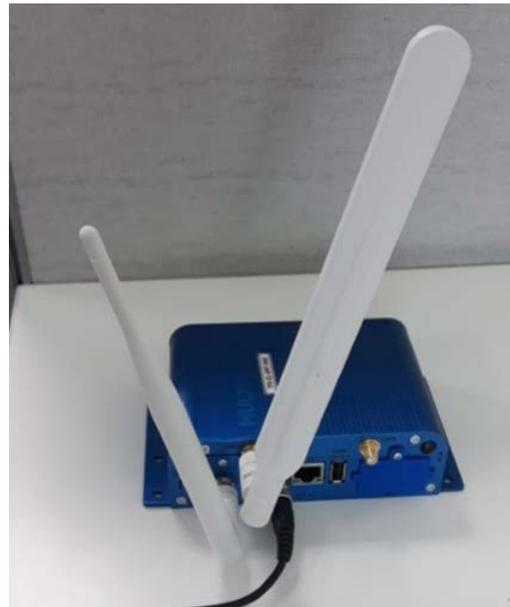
**Figure 24. Attaching antenna for Wi-Fi network**
