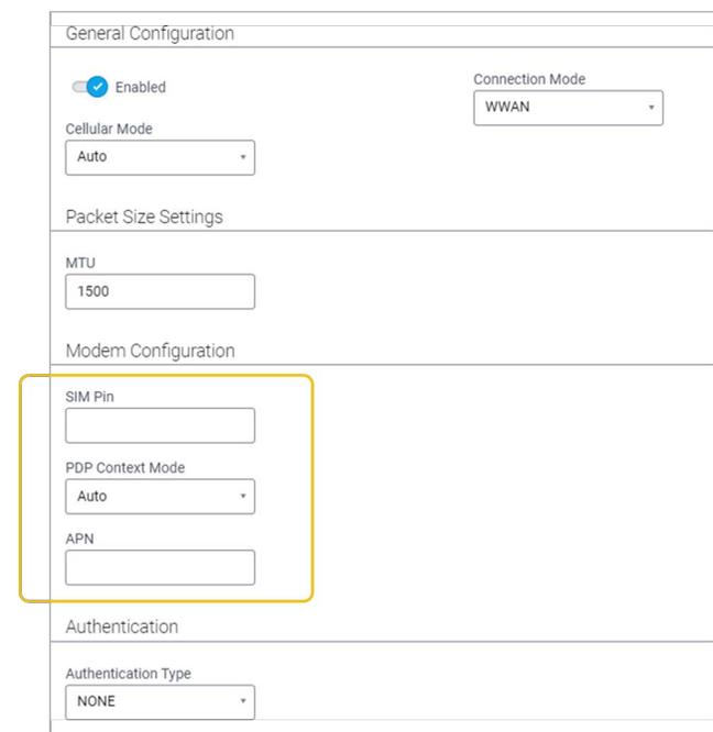
**Figure 32. Cellular configuration interface**
