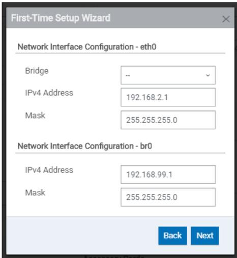
**Figure 19. Network interface configuration**
