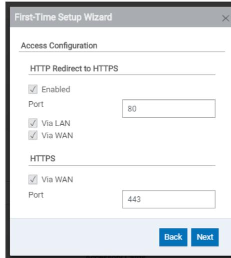
**Figure 20. Access configuration**
