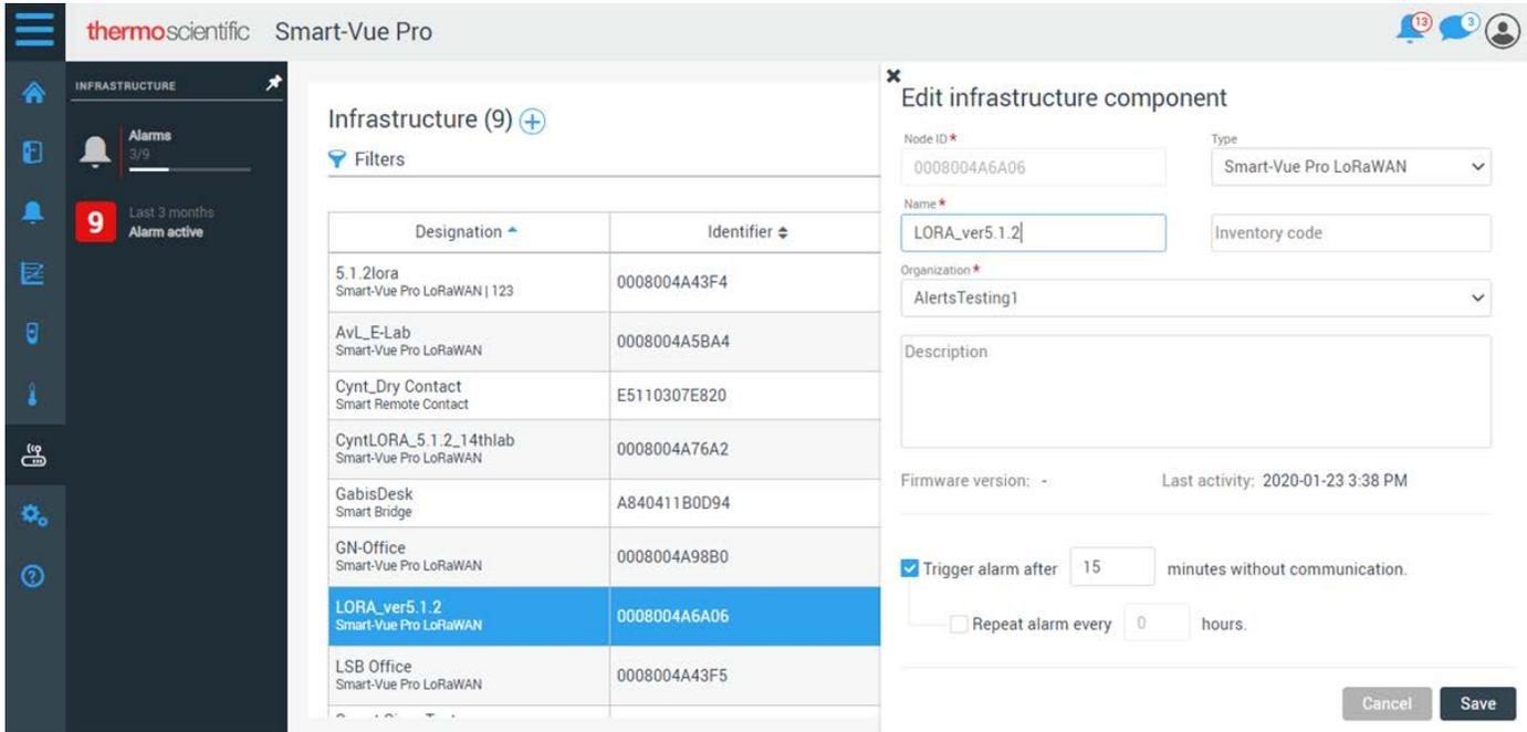
**Figure 48. Add the node ID in Smart-Vue Pro LoRaWAN label**
