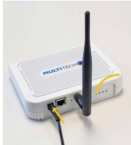
**Figure 10. Plug in the power cable into the power plug and wait for the LED to turn green**
