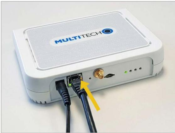
**Figure 12. Pro model receiver with ethernet cable**
