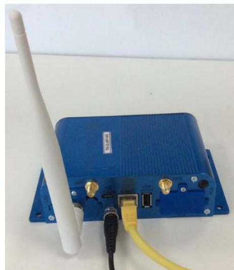
**Figure 11. Advanced model receiver with ethernet cable**
