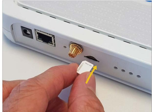
**Figure 31. Insert the SIM into the gateway**
