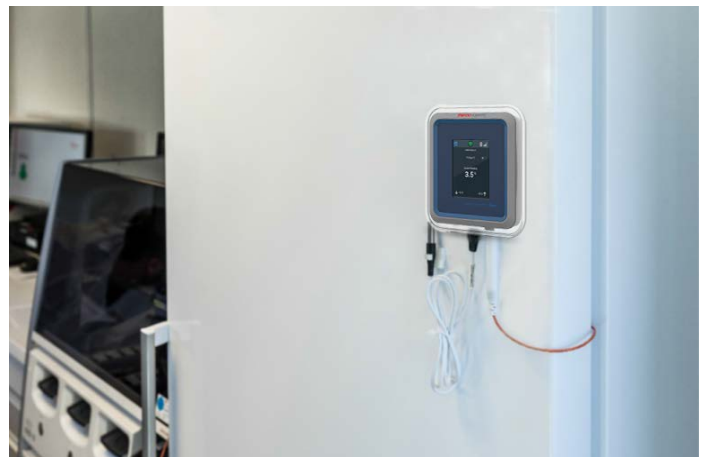
Figure 24. Smart-Vue Pro Duo/Quatro data logger mounted on the refrigerator door
