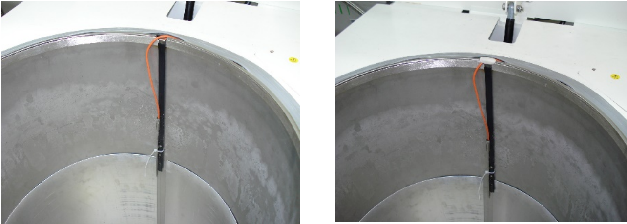
Figure 20. Pt100 (-200 °C to + 50 °C) for nitrogen/cryogenic tank
