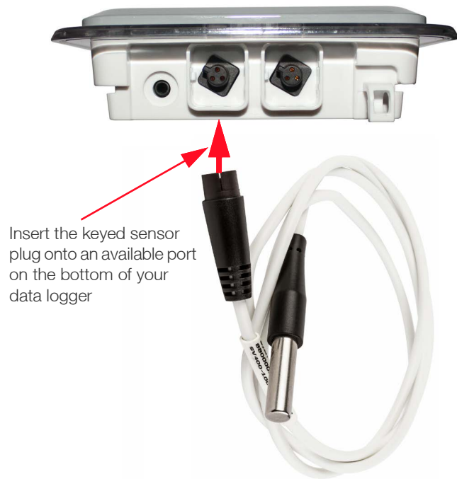
Figure 22. Smart-Vue Pro Duo/Quatro data logger with external digital sensor
