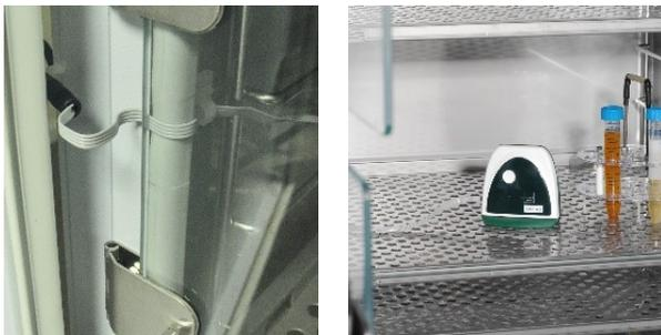
**Figure 21. Ribbon cable connecting to sensor unit inside incubator**
