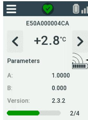
Wireless icon indicates that the sensor is a wireless remote sensor
