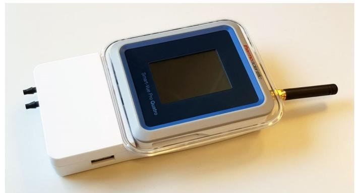
**Figure 38. Slide the smart sensor extension onto Smart-Vue Pro data logger**
