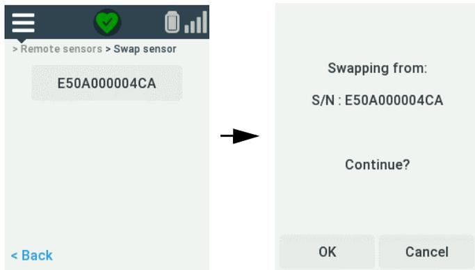
**Figure 12. Choose the current wireless remote sensor you want to replace**
