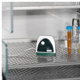
**Figure 25. Sensor unit inside incubator**
