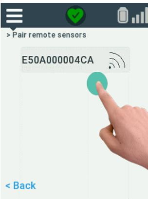
**Figure 8. Tap to pair the wireless remote sensor**
