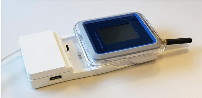
**Figure 26. Slide the Smart-Vue Pro data logger onto the extension cradle**
