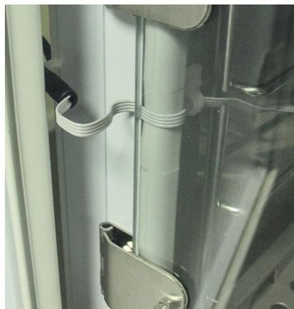
**Figure 24. Ribbon cable lays flat beneath door joint**
