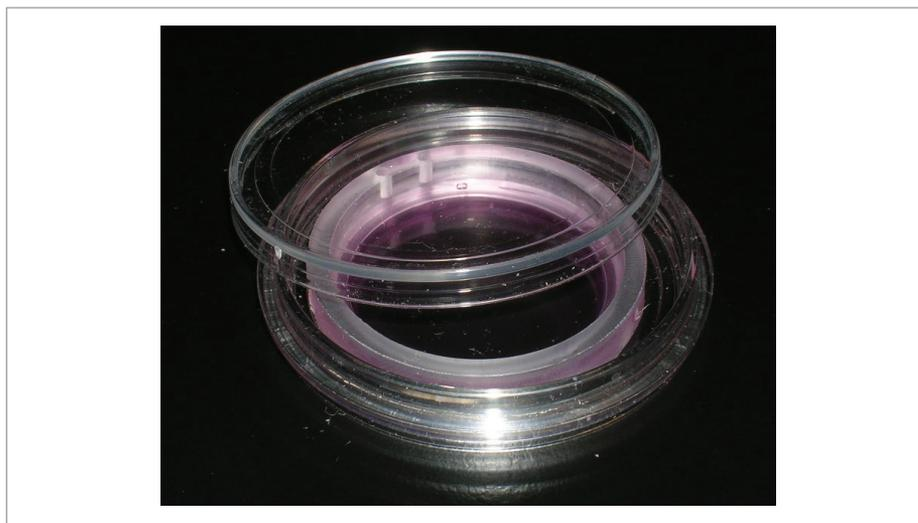
**Figure 4. Arcturus<sup>x7™</sup> Live Cell Growth Chamber/Microdissection Dish Assembly with Media.** Once the Arcturus<sup>x7™</sup> Live Cell Growth Chamber has been placed into the Arcturus<sup>x7™</sup> Microdissection Petri Dish, the entire assembly is carried to the Arcturus<sup>x7™</sup> Microdissection Instrument. With the lid on the Arcturus<sup>x7™</sup> Microdissection Petri Dish, sterility is maintained throughout the microdissection experiment.
