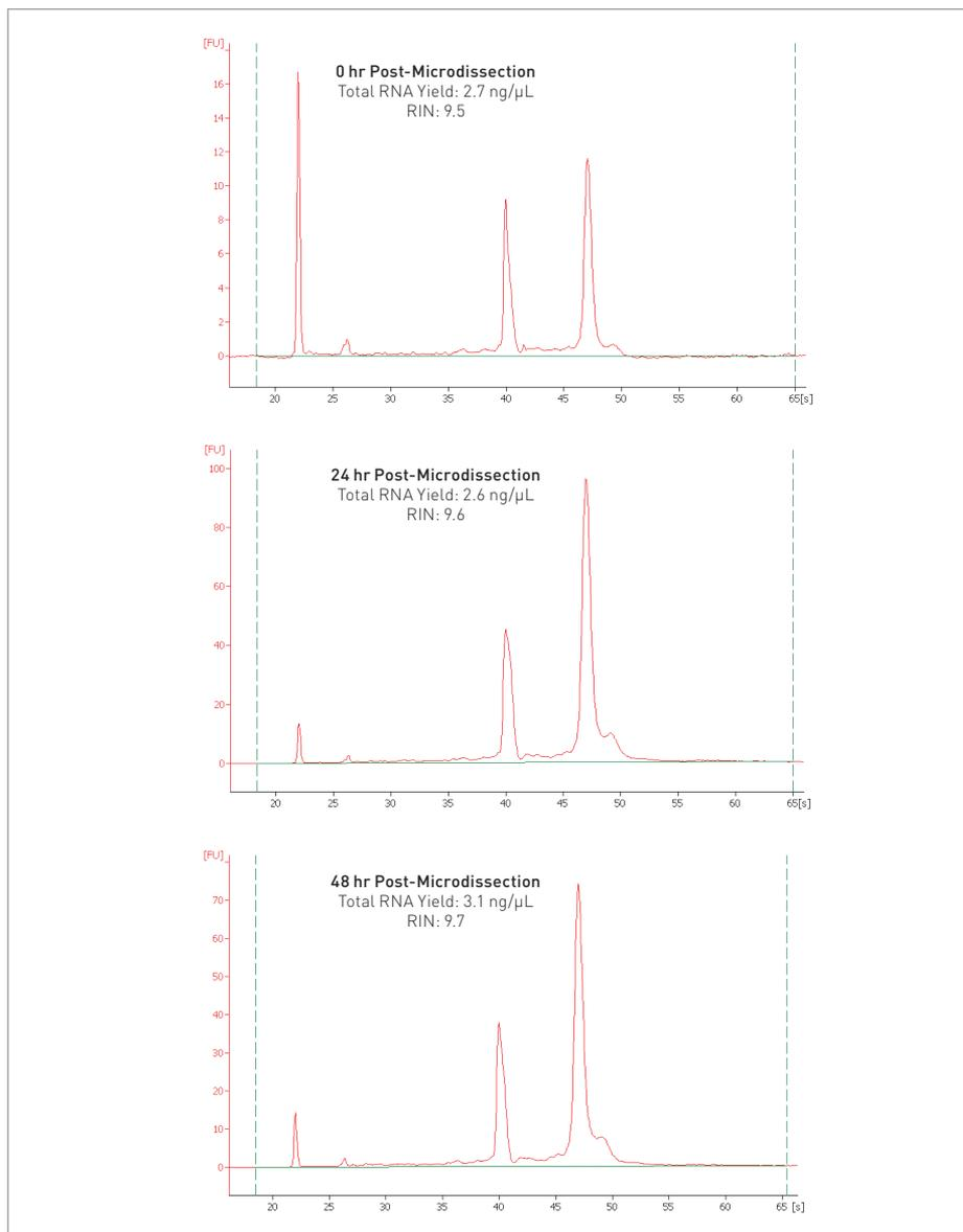
**Figure 7. Total RNA Assessment, Post-Microdissection.** Live cells were microdissected using the Arcturus<sup>XTM</sup> LCM instrument, and total RNA was isolated at 0 hr, 24 hr, and 48 hr post-microdissection. Total RNA quality (Agilent Bioanalyzer) and total RNA yield (NanoDrop<sup>®</sup> ND-1000) were measured, both demonstrating that the microdissection process does not damage the RNA.
