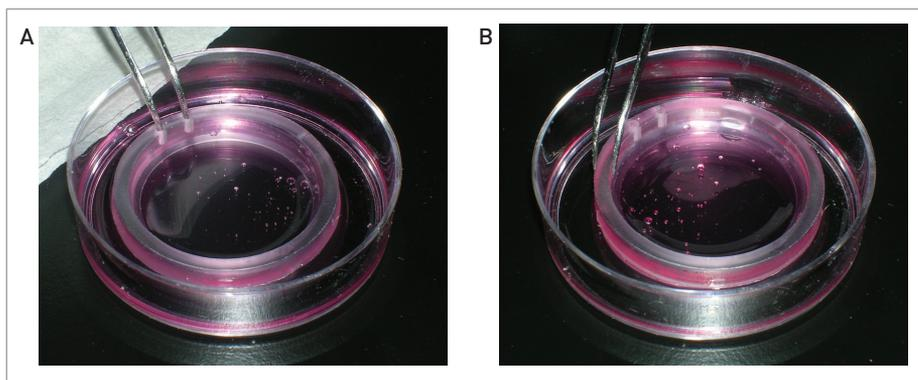
**Figure 3. Removing Arcturus<sup>x7™</sup> Live Cell Growth Chamber from Petri Dish.** Under sterile conditions, the Arcturus<sup>x7™</sup> Live Cell Growth Chamber is carefully removed from the standard petri dish for transfer to the Arcturus<sup>x7™</sup> Microdissection Petri Dish.
