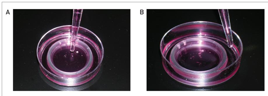
**Figure 2. Cell Culture in the Arcturus<sup>x7™</sup> Live Cell Growth Chamber.** Live cells are seeded directly onto the PEN membrane of the Arcturus<sup>x7™</sup> Live Cell Growth Chamber, which is placed inside a standard petri dish. Media is added to both the Arcturus<sup>x7™</sup> Live Cell Growth Chamber and to the surrounding petri dish to facilitate cell growth.
