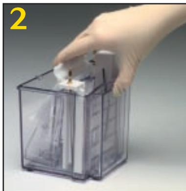
Lock the gel tension wedge in place, load samples, and fill the buffer chambers with the appropriate running buffers.
