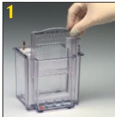
Drop buffer core into the lower buffer chamber of the XCell *SureLock™* Mini-Cell, insert one mini-gel in front of the buffer core and a second mini-gel or the buffer dam behind the buffer core.
