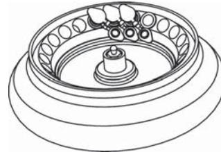
**!** *To avoid potential breakage of the microcentrifuge tube cap during centrifugation, insert the purification column/ 0.5 mL tube assembly into a lidless 1.7/2.0 mL tube. Insert this assembly into adjacent rotor holes as illustrated. Rest the tube cap against the tube immediately clockwise to it. Place an empty, lidless 1.7/2.0 mL tube into the rotor hole adjacent in the clockwise direction to the last assembly.*
