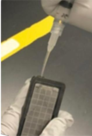
The syringe tip must be in front of the array when filling the case with immersion fluid.
