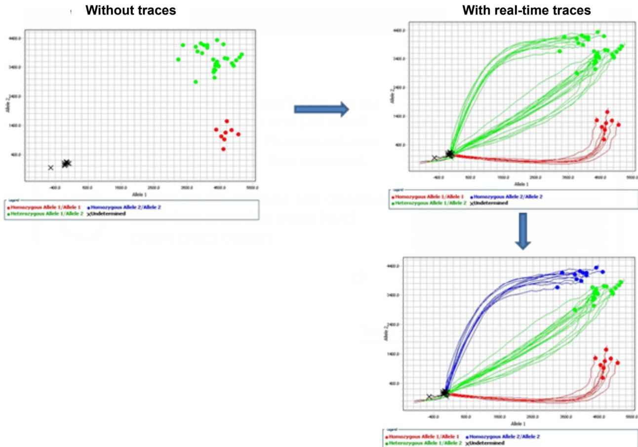
Left: Calls based on end-point reads could be incorrect. Right: Real-time genotyping graphs used for making accurate calls when using samples with very high DNA concentration. Red: homozygous Allele 1/Allele 1. Blue: homozygous Allele 2/Allele 2. Green: heterozygous Allele 1/Allele 2.
