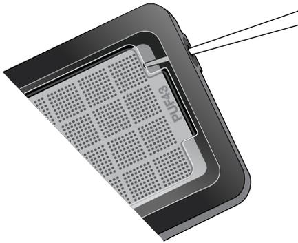
9. Slowly inject the OpenArray™ Immersion Fluid until the case is filled, which should take about 10 seconds to fill. Minimize the creation of additional air bubbles when you dispense the fluid. Leave a small air bubble as shown below.
