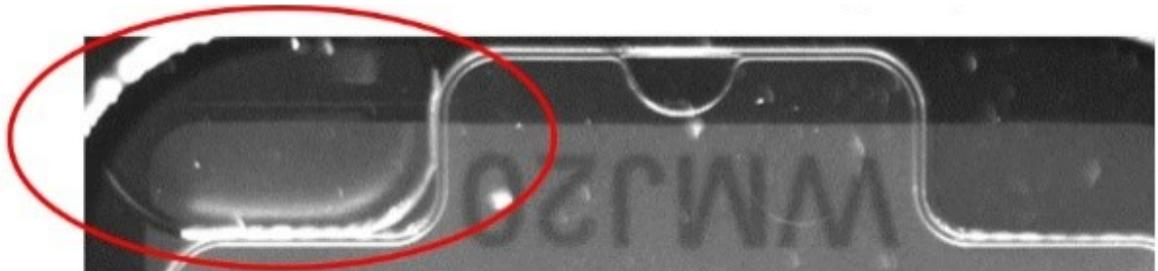
10. While holding the case *vertically*, remove the syringe tip, insert the screw end of the OpenArray™ plug into the port of the case, then rotate clockwise until the black handle breaks off.
