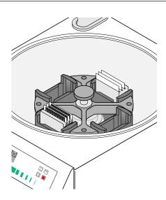
Centrifuge is properly loaded and balanced.
