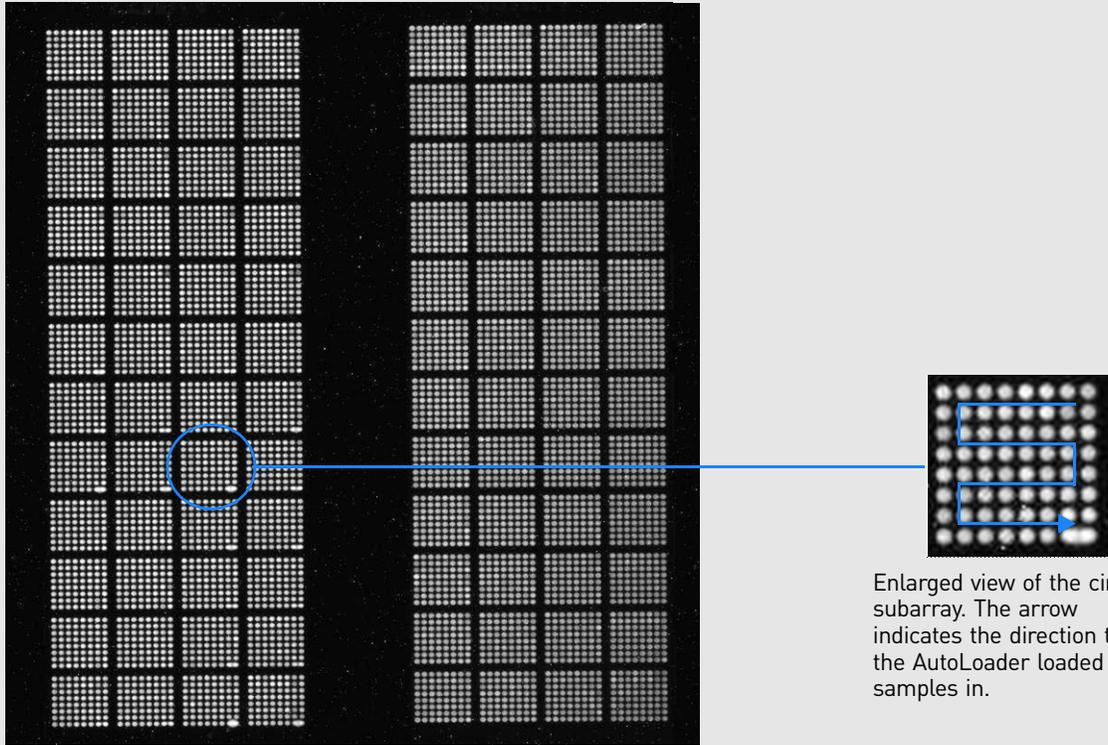
Enlarged view of the circled subarray. The arrow indicates the direction that the AutoLoader loaded the samples in.
