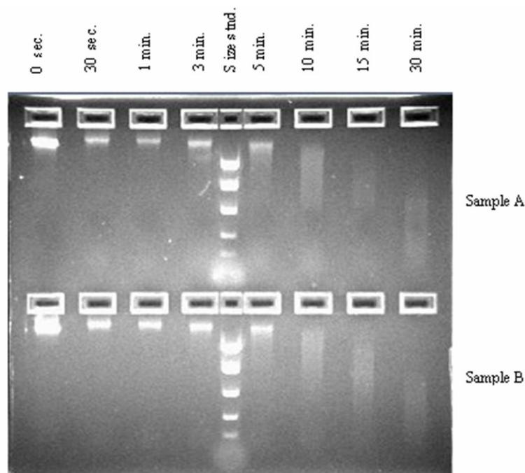
The scatter plots shown below illustrate the effects of DNA degradation caused by heating.
