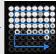
Enlarged view of the circled subarray. The arrow indicates the direction that the AutoLoader loaded the samples in.
