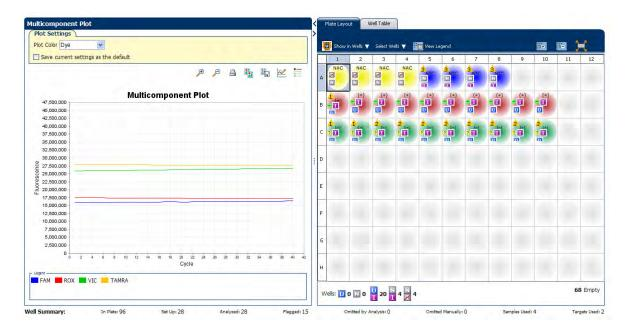
9. Select the negative control (NTC) wells one at time and check for amplification. In the example experiment, there is no amplification in the negative control wells.
