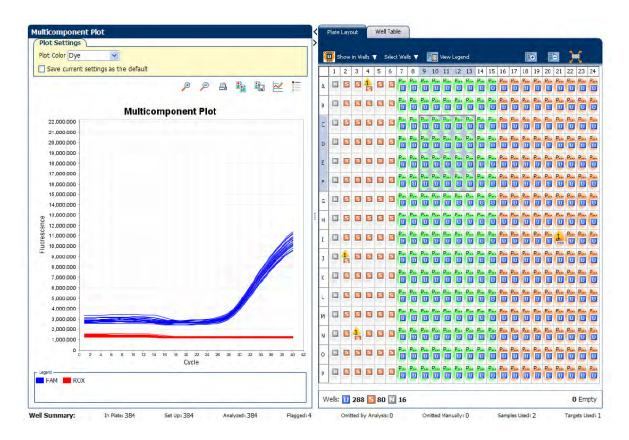
7. Select the negative control wells one at time and check for amplification.
