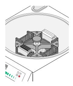
8. When the second run is finished, open the centrifuge and check that the fluid levels in the reservoirs of each array card have decreased by the same amount. Also, check for the formation of bubbles in all wells and note possible problems.
