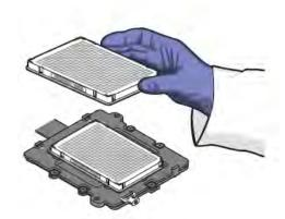
• If using reaction tubes or tube strips, make sure you use adaptors. The adaptors are attached to the plate transport arm. The tray containing the tubes or tube strips must be placed on the adaptor and not into the sample block directly.
