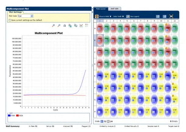
6. Select the negative control wells one at time and check for amplification.
