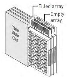
5. Place the filled carrier clips into the centrifuge buckets. Make sure that the array-card fill reservoirs and bucket and clip labels face outward when loaded into the centrifuge. Balance the loads in opposite buckets.
