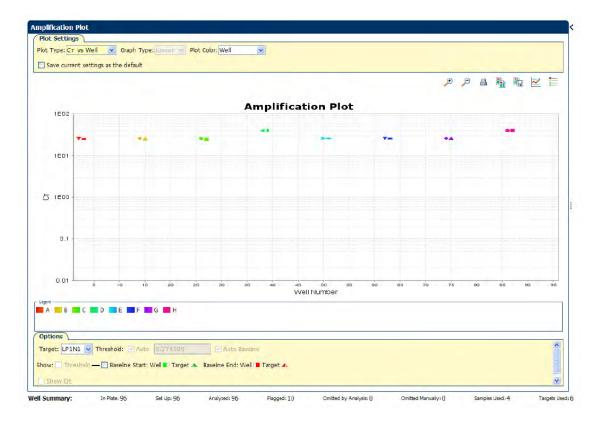
7. Repeat step 2 to step 6 for the GH1, TGFB1, LIPC, ACTB, and CCKAR wells. In the example experiment, there is seven outliers for CCKAR and three outliers for GH1. These wells are omitted in the troubleshooting section ("Improve CT precision by omitting wells" on page 248).
