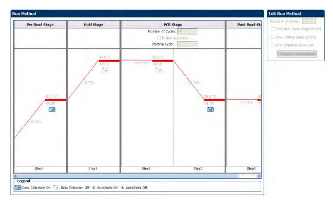
Figure 101 The Run Method screen as it appears in the example experiment
