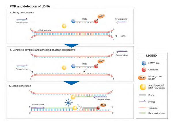
Figure 1 TaqMan™ reagents detection process
