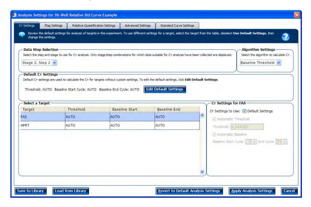
Figure 48 Analysis Settings dialog box for a Relative Standard Curve experiment
