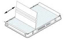
6. Using the applicator to hold the edge of the film in place, grasp one end of the end-tab and pull up and away sharply. Repeat for the other end-tab.
