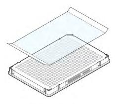
Applying firm pressure, move the applicator slowly across the film, horizontally and vertically, to ensure good contact between the film and the entire surface of the reaction plate.
