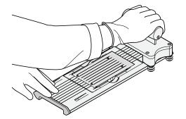
5. Remove the sealed array card from the fixture and trim the fill reservoirs from the array card assembly using scissors. Trim the foil array card so that the edge is even with the plastic carrier.
