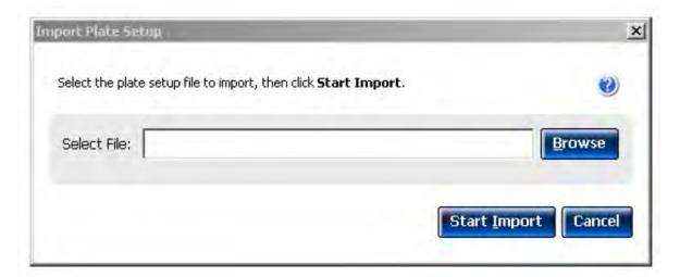
4. Click **Start Import**. The setup data from the exported text file is imported into the open experiment.
