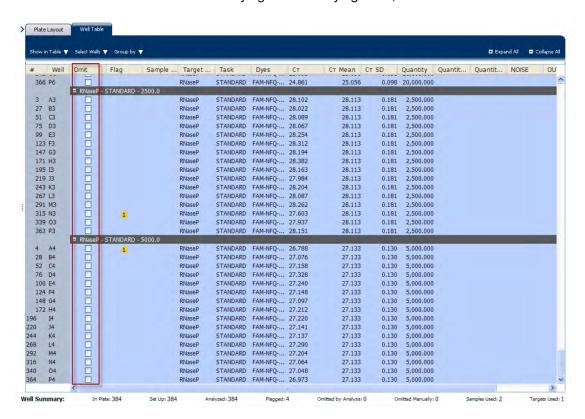
5. Click **Analyze** to reanalyze the experiment data with the outlying well or outlying wells removed from the analysis.
