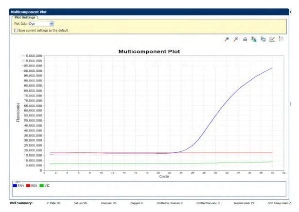
7. Select the no template control wells one at time and check for amplification.
