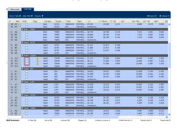
5. Click **Analyze** to reanalyze the experiment data with the outlying well or outlying wells removed from the analysis.
