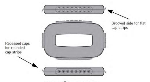
MicroAmp® Cap Installing Tool
