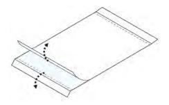
4. Holding the film by the end-tabs, lower the film onto the reaction plate (adhesive side facing the reaction plate). Make sure that the film completely covers all wells of the reaction plate.
