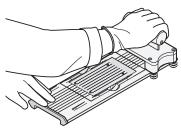
e. Remove the sealed array card from the fixture and trim the fill reservoirs from the array card assembly using scissors. Trim the foil array card so that the edge is even with the plastic carrier. Completely remove the fill reservoirs from the array card so that the edge is free of residual plastic. The plastic from the fill reservoirs that extends beyond the edge of the card can prevent the card from seating properly on the sample block and affect amplification.
