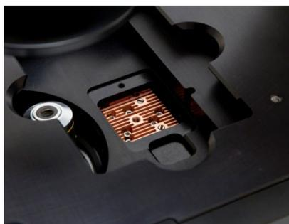
5. Screw the threaded end of the light cube tool into the hole in the center of the light cube as shown.
