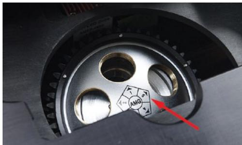
2. Screw the new objective into the open position in the objective turret. Note the part number of the objective and the turret position.
