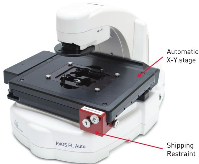
1. Unscrew the three thumb screws until they spin freely. You do not need to remove them from the shipping restraint altogether.
