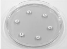
Precision positioning of discs equally spaced on 54mm circle.
