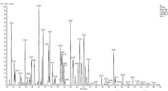
Base peak chromatogram of 40 ug BSA Digest separated using a Thermo Scientific<sup>TM</sup> Acclaim PepMap<sup>TM</sup> RSLC, C18, 3  $\mu$ m, 100Å, 75 $\mu$ m x 15cm column (P/N ES900) with 2-25% gradient (A: 0.1% FA in water, B: 0.1% FA in 100% acetonitrile) at 300 nL/min and detected on a Thermo Scientific<sup>TM</sup> Orbitrap<sup>TM</sup> Eclipse Mass Spectrometer.
